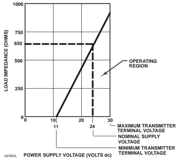
**Figure 3. Transmitter Load Limitations**
